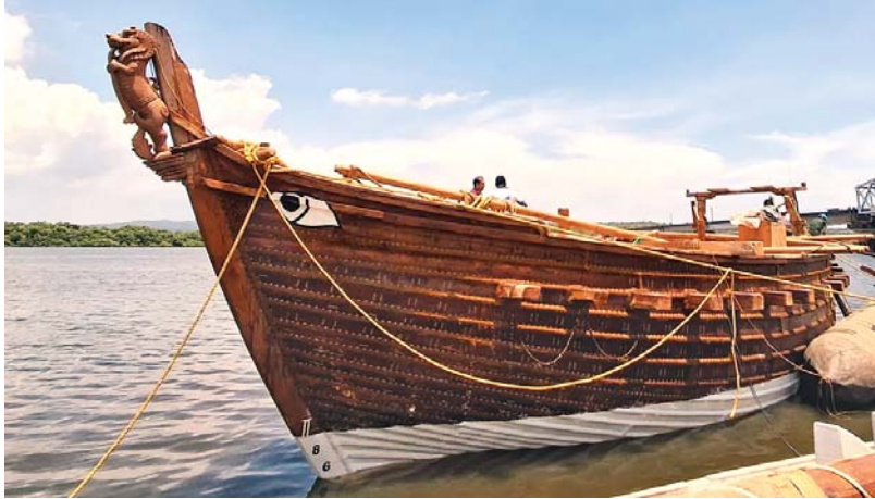
A naval ship made in the ancient tradition of no nails used.
