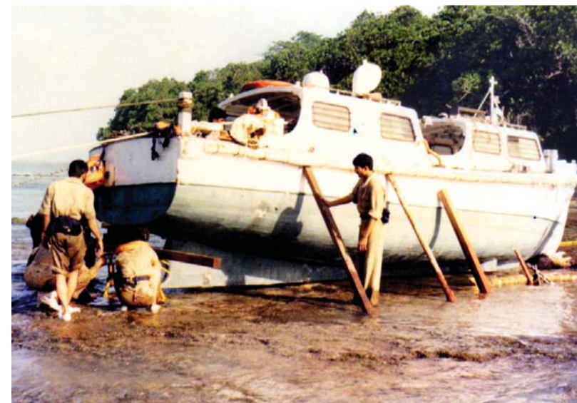
Boat aground with shoring to prevent toppling.
