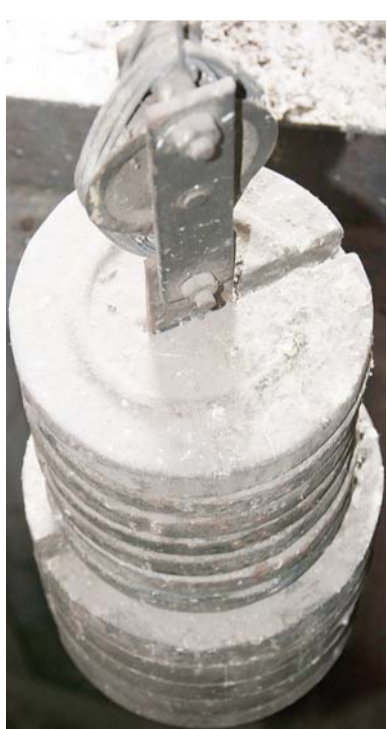
The driving weight comprises of two different sizes of separate cast iron weight plates. Back in the day, this led to the speeding up or slowing down of the escapement.
