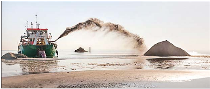
A Dredger creating an island from dredged material.
